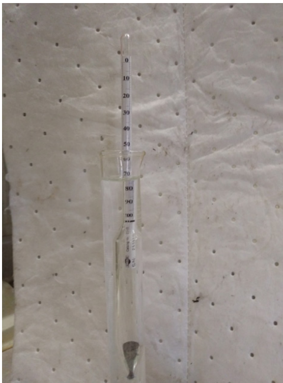
Figure 3 – Hydrometer Measuring NaCl Solution
