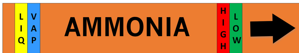
Figure 13 – Ammonia Piping Label
