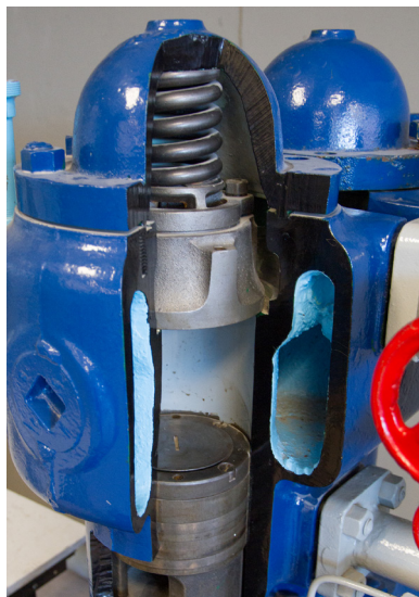
Figure 5 – Compressor Showing Valve Assembly with Safety Spring
