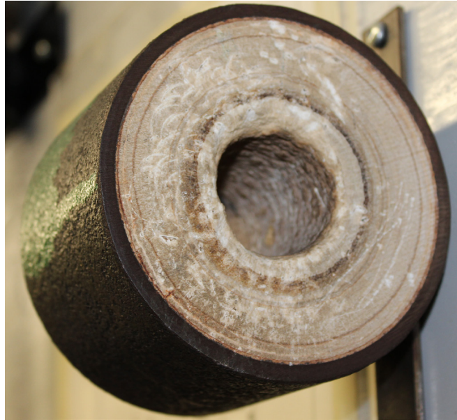
Figure 3 – Solid Scale Inside a Tube
