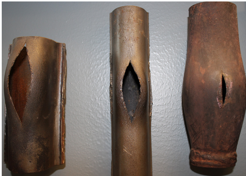
Figure 4 – Tubes Damaged from Overheating
