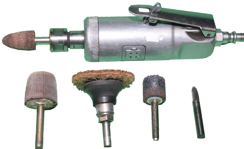
(b) Pneumatic die grinder with attachments
