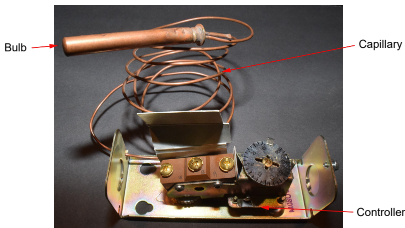
Figure 4 – Remote Bulb Thermostat
