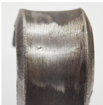
1. Cleaned, ready for dye penetrant
