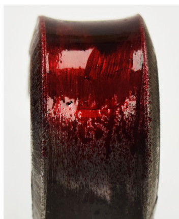
2. Dye penetrant applied
